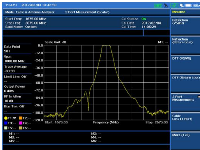
Cable and antenna test — 2-port Measurement
