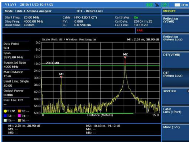
Cable and antenna test — Distance to Fault
