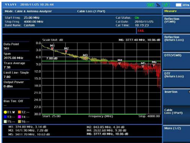
Cable and antenna test — Cable Loss
